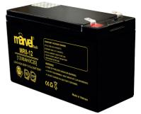
MR series is a general purpose battery with 6~8 years design life in float service. It meets with IEC, JIS, BS, GB/T and YD/T standards. With advanced AGM valve regulated technology and high purity raw material, the MR series battery maintains high consistency for better performance and reliable standby service life. It is suitable for UPS/EPS, medical equipment, emergency light and security system applications.
