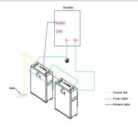
**Battery Packs Connected in Parallel**
