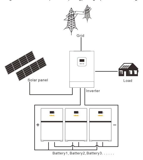
Figure 1 Operation Principle Diagram of Battery System
