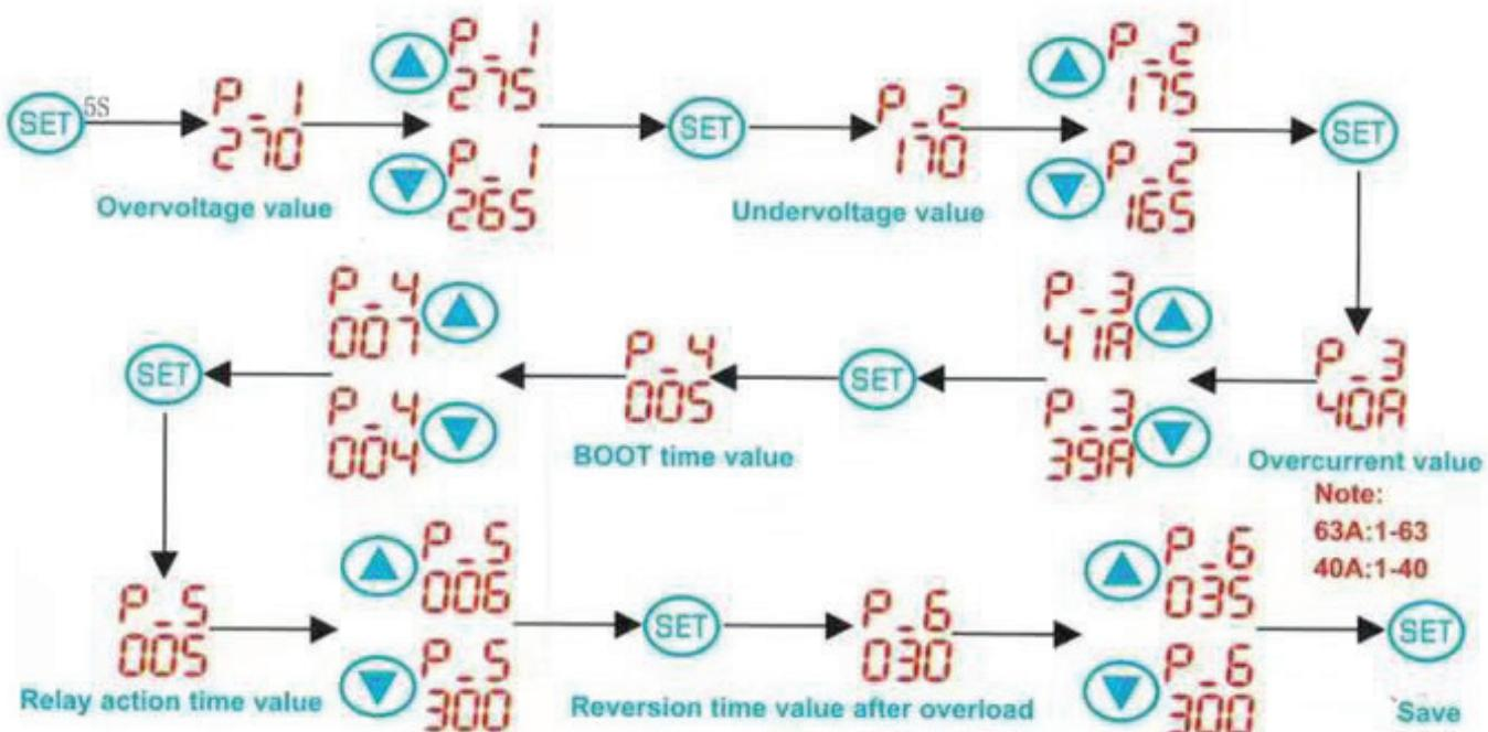
Note: If the keyboard is no longer than 60 seconds at any location before saving, the operating system will abandon all settings and restart.
