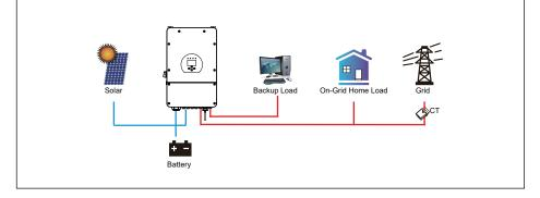
**Solar Sell:** "Solar sell" is for Zero export to load or Zero export to CT: when this item is active, the surplus energy can be sold back to grid. When it is active, PV Power source priority usage is as follows: load consumption and charge battery and feed into grid.
