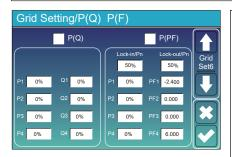
P(Q): It is used to adjust the inverter reactive power according to the set active power. P(PF): It is used to adjust the inverter PF according
