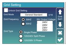
**Unlock Grid Setting:** before changing the grid parameters, please enable this with password of 7777. Then it is allowed to change the grid parameters.
