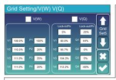
V(W): It is used to adjust the inverter active power according to the set grid voltage.
