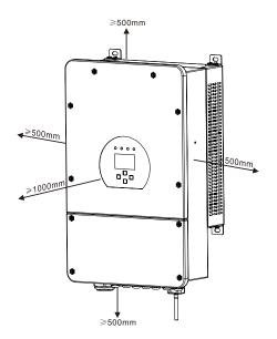
For proper air circulation to dissipate heat, allow a clearance of approx. 50cm to the side and approx. 50cm above and below the unit. And 100cm to the front.
