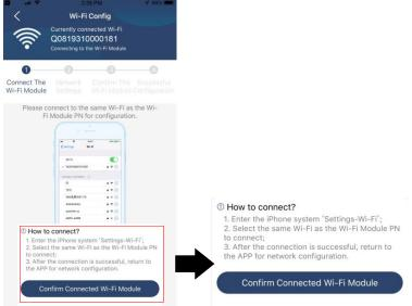
Enter the "Settings→Wi-Fi" and select connected Wi-Fi name. The connected Wi-Fi name is the same to your Wi-Fi PN number and enter default password "12345678".
