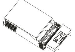
Step 2: Remove two screws as below chart and remove 2-pin and 14-pin cables. Take out the board under the communication board.
