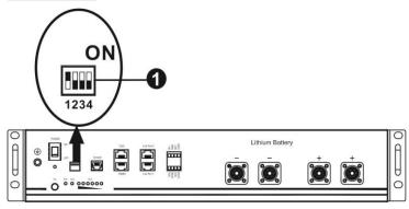
• ADD Switch: There are 4 ADD switches are to define different baud rate and battery group address. If switch position is turned to bottom for "OFF" position, it means "0". If switch position is turned to upper for "ON" position, it means "1".
