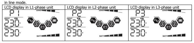
Step 5: If there is no more fault alarm, the system to support 3-phase equipment is completely installed.
