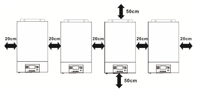
**NOTE:** For proper air circulation to dissipate heat, allow a clearance of approx. 20 cm to the side and approx. 50 cm above and below the unit. Be sure to install each unit in the same level.
