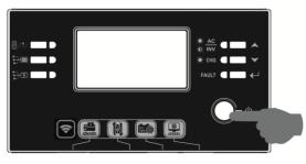
Step 4. Be sure to select battery type as "SOL" in LCD program 5.
