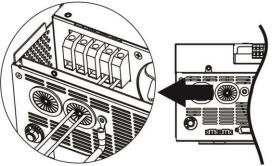
5. Make sure the wires are securely connected.
